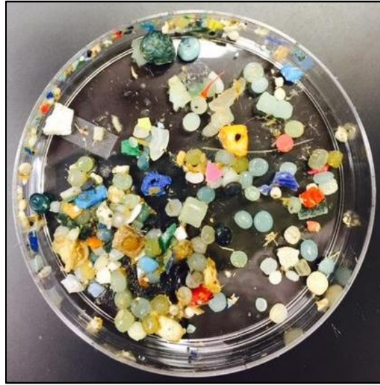
Figure 10. Plastic sample collected from Newark Bay exhibited pre-production pellets (nurdles) and microplastic fragments. The smallest particles counted were approximately the size of a grain of sand.
