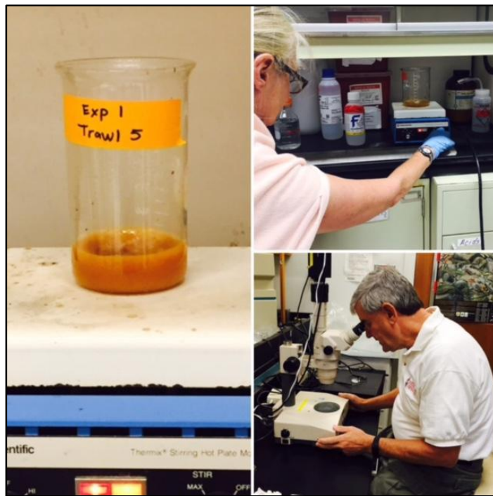
Figure 9. Samples undergoing oxidation digest and examination under microscope.
