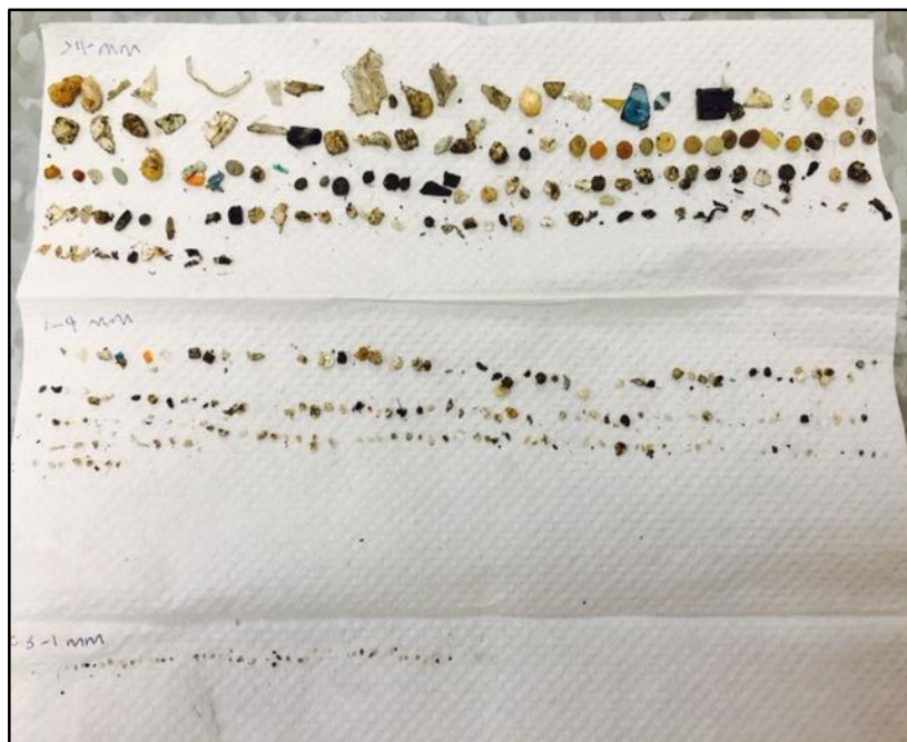
Figure 12. Plastics separated into size categories three size classes (0.355-0.999 mm, 1.00-4.749 mm, and >4.75 mm) after counting.
